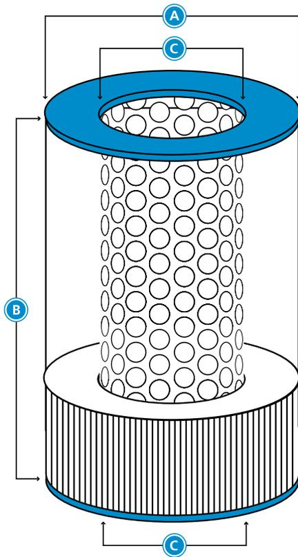
The Filbur Catalog for replacement cartridges is divided into two sections, Dimensional and Pool/Spa OEM. The cartridges are listed alphabetically by original manufacturer, and then each cartridge for that manufacturer is listed from the smallest O.D. (outside diameter) to the largest, then by overall length, top (measurement or handle, etc.), bottom diameter, and description (manufacturer).
